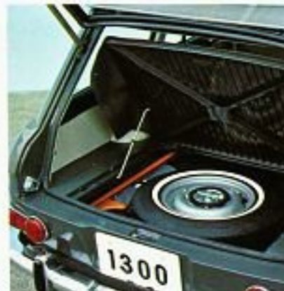
Spare tire is neatly stored beneath the floor of luggage compartment.
